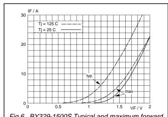
Fig.6. BY329-1500S Typical and maximum forward characteristic  $I_F = f(V_F)$ ; parameter  $T_j$
